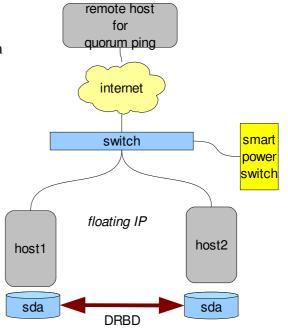
The SAN could be setup with a non-clustered or a clustered filesystem, the difference being that a clustered filesystem is required if you require both servers to be able to run services at once
